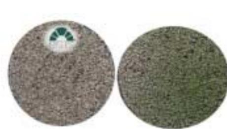
Roofing Shingles treated with the ÆGIS Microbe Shield technology (left) show no algal growth as compared to an untreated shingle.
