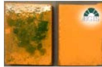
Laboratory testing proves roofing tiles treated with the ÆGIS Microbe Shield technology significantly control algal and fungal growth.
